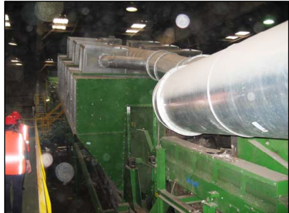
Figure 3.11: Nihot Drum Separator
