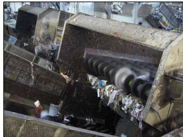
Figure 3.19: Disk Screen at WPWMA
